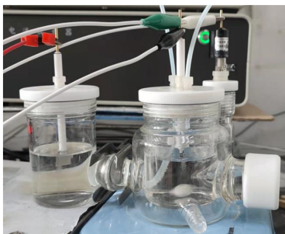
Figure S10. Photograph of the H-cell containing 180 mL of 0.5 M KHCO 3 with two compartments separated by the Nafion 117 membrane.
